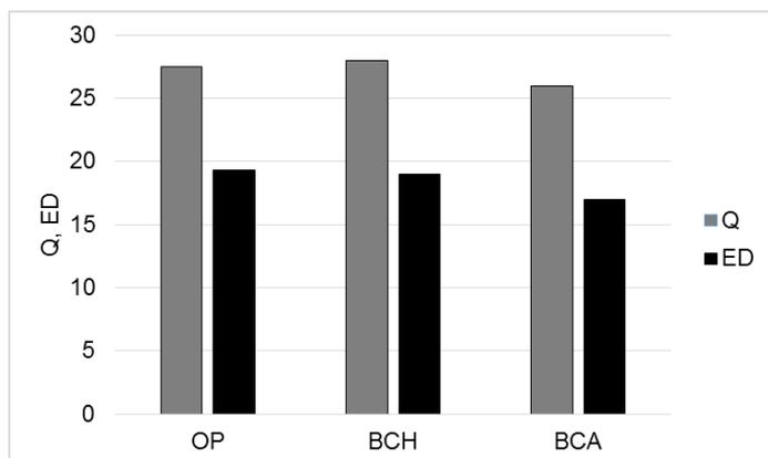
**Figure 1.** Fuel characteristics of OP pellets coated with PB (OP) in comparison with bituminous coal of high quality (BCH) and average quality (BCA)
