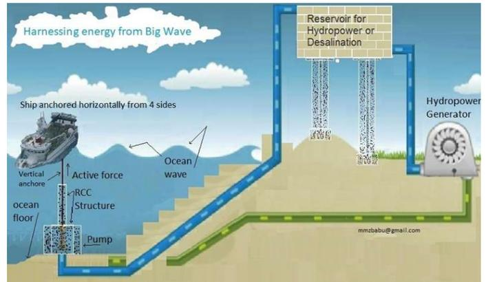
Figure 7: Vertical force of Tidal waves are pumping water to reservoir.
