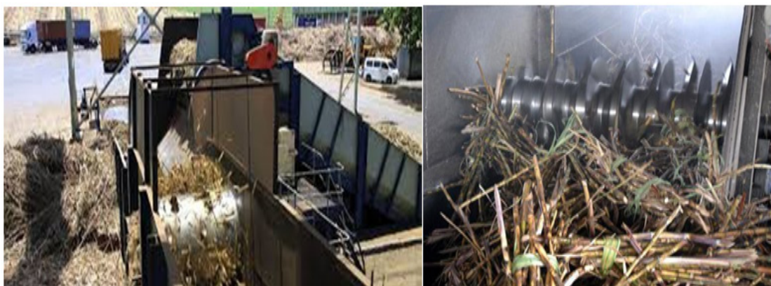
Figure 2: Sugarcane carrier and cutter blades
